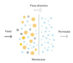
When the electrophoretic paint passes through the membrane, the polymer resin and color paste are intercepted, and water and small molecule substances are allowed to pass, thereby achieving the purpose of purifying the electrophoretic paint and dewatering.
